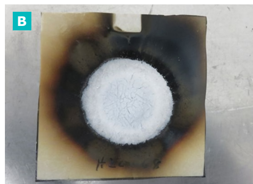
Figure 20: UP-laminate (15 wt.-% GF) after torch test: A) 300 phr APYRAL® HC 500 and B) 200 phr ACTILOX® HTB .
